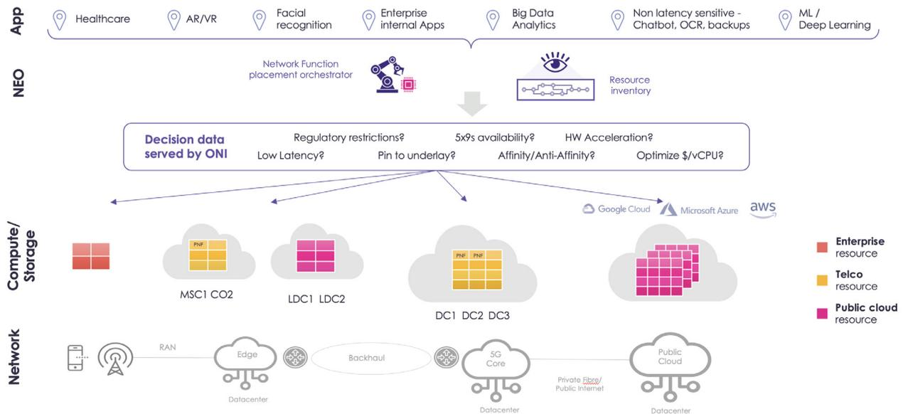
Figure 2: 5G Network Function Placement
