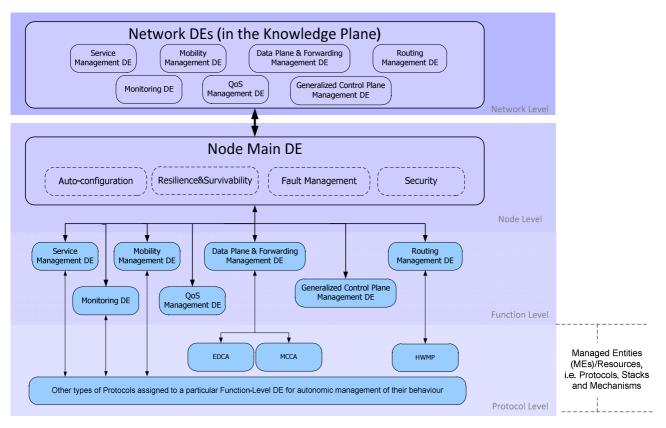
Figure 8: Complementary Views on Block diagram of DEs in autonomicity-enabled Ad-hoc and mesh architecture
