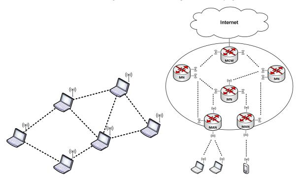
Figure 7: Common aspects between Ad-hoc (*left*) and mesh networks (*right*) include multi-hop wireless transmission
