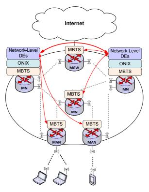
Figure 10: Overlay Knowledge Plane in a mesh network
